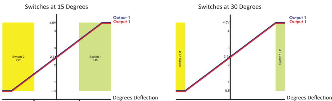
Note: When Dual Output (non-inverted) option is selected the polarity of Switch 2 is inverted
