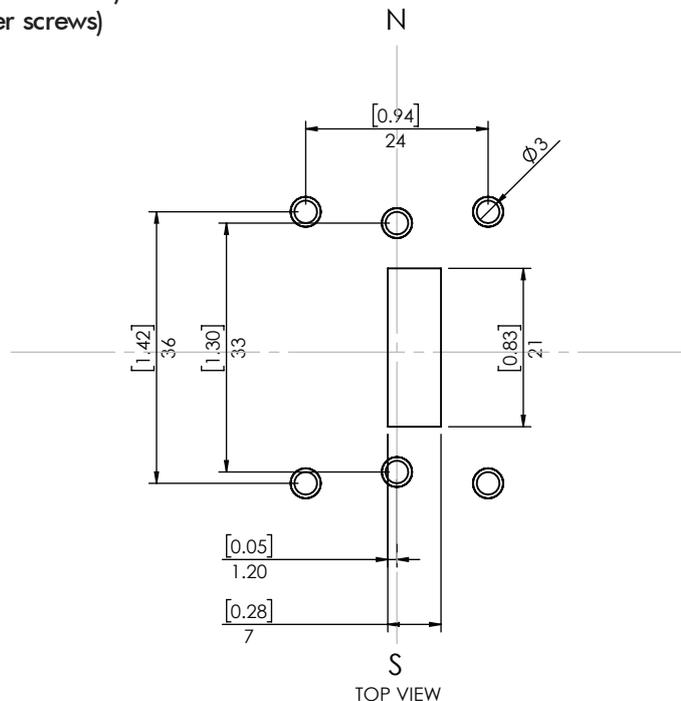
The Paddle is fitted with M3 bushes in all six positions, as standard.
